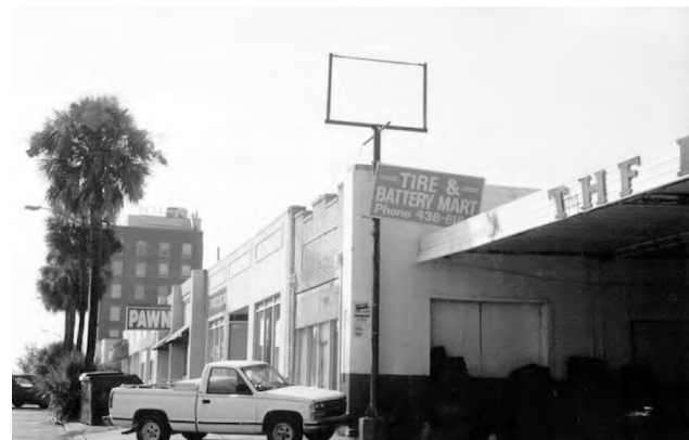
✗ This pole-mounted sign is not at an appropriate scale for the surrounding one-story, commercial buildings. A more appropriately-designed sign would be no taller than the roofline of the surrounding buildings.
