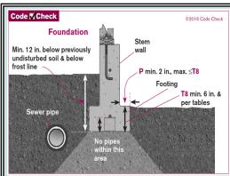
Foundation bottom must be 12" below undisturbed soil
